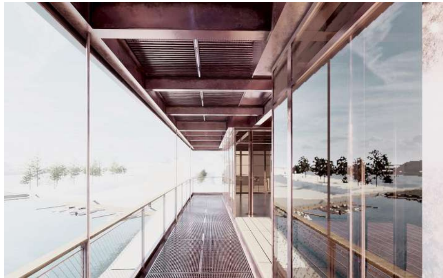
peripheral walkway floor structure made of steel grating
